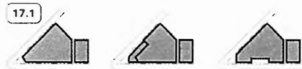
✓ Figure 68. Acceptable examples of curved or angled planes used in a subordinate manner
